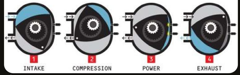
Disadvantages of the Wankel engine include imperfect sealing against the chamber ends, which counts for leakage between adjacent chambers, and unburned fuel mixture. The rotary combustion engine also has a 50% longer stroke duration compared to a piston engine. The engine's operation also allows for more carbon monoxide and unburned hydrocarbons in the exhaust stream, making it an obvious pariah among tree-huggers.
