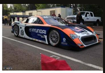
The car is powered by a 671kW turbocharged version of Hyundai's 4.1-litre V6 engine that belts out a spleen-smashing 1085Nm of torque. The force-fed mid-mounted six-cylinder engine drives through a five-speed sequential gearbox, and the whole kit and caboodle weighs 861kg.
